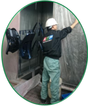
Tacky surface coating / for catching dusty
